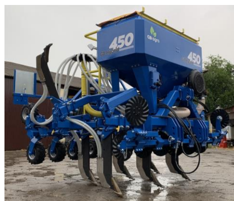
GB Hybrid- Strip-till and subsoiler
